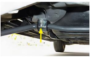
8. Remove the 18mm nuts from the lower end links. It may be necessary to hold the hex on the bolt end with an 8mm wrench if the bolt spins during removal. The original nuts will be used for installation.
